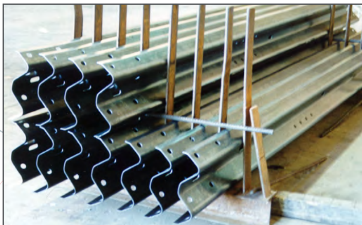
Proper storage of galvanized steel to avoid wet storage stain
