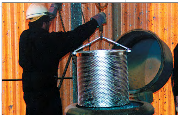
A perforated basket filled with bolts is placed in a centrifuge to spin off excess zinc
