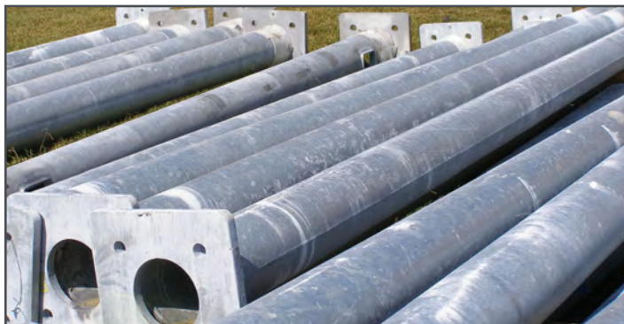
Poles with wet storage stain
