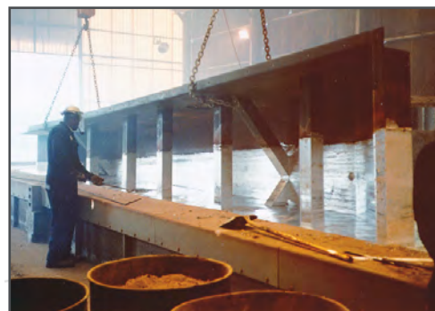
Progressive dipping - galvanizing oversized pieces
