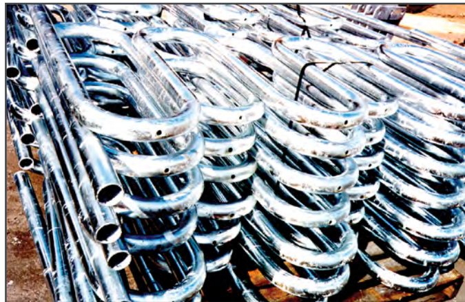
Hot-dip galvanizing cold-worked steel is very successful when following suggested guidelines
